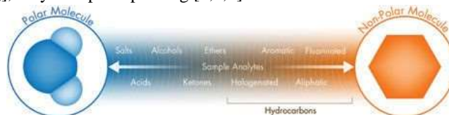
Compound/Analyte Chromatographic Polarity Spectrum
