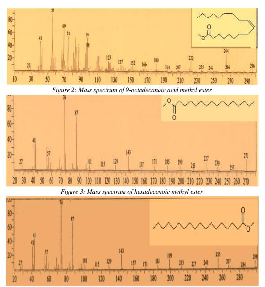
Figure 4: Mass spectrum of methyl stearate
