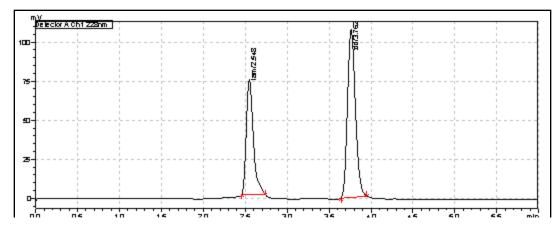
Figure 4: Chromatogram showing resolved peaks of LAM and ZID
