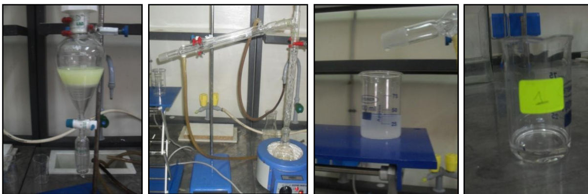
Figure 2: Washing, distillation and recovery of benzyl alcohol at T = 205\text{ }^{\circ}\text{C} .
