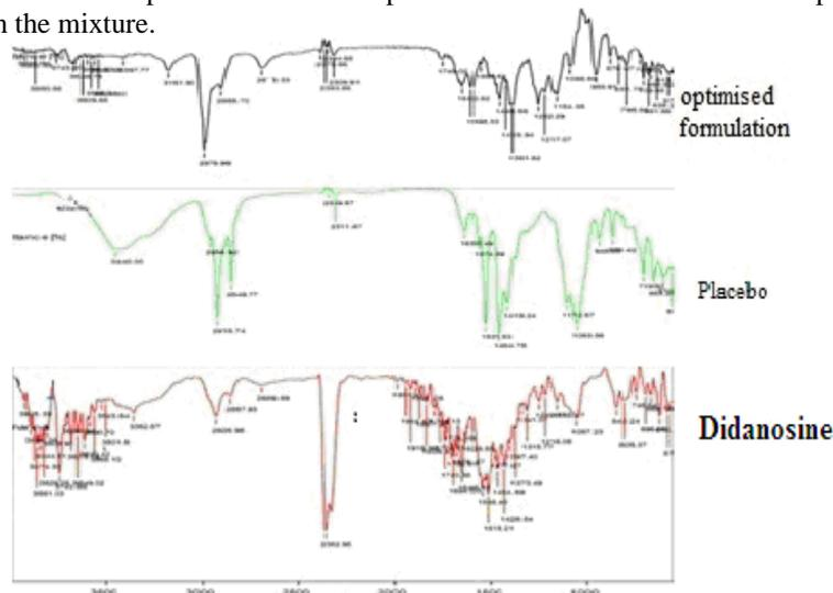
Figure 4: Ftir Studies For The Pure Drug, The Optimized Didanosine Enteric Coated Tablet Formulation And Placebo
